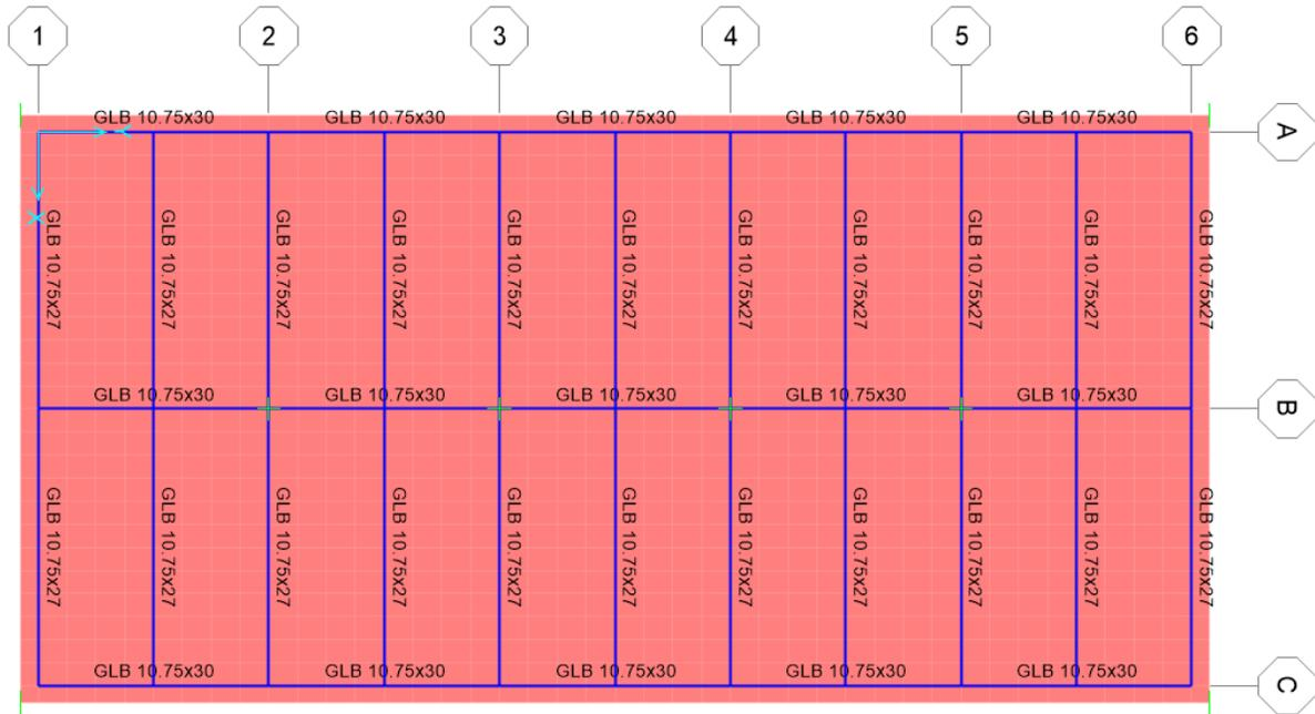
**FIGURE 9-2** Floor plan showing framing; CLT3 spans left to right
