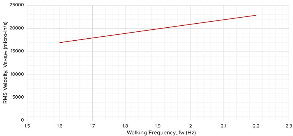
**FIGURE 8-6:** Transient velocity response vs. walking frequency
