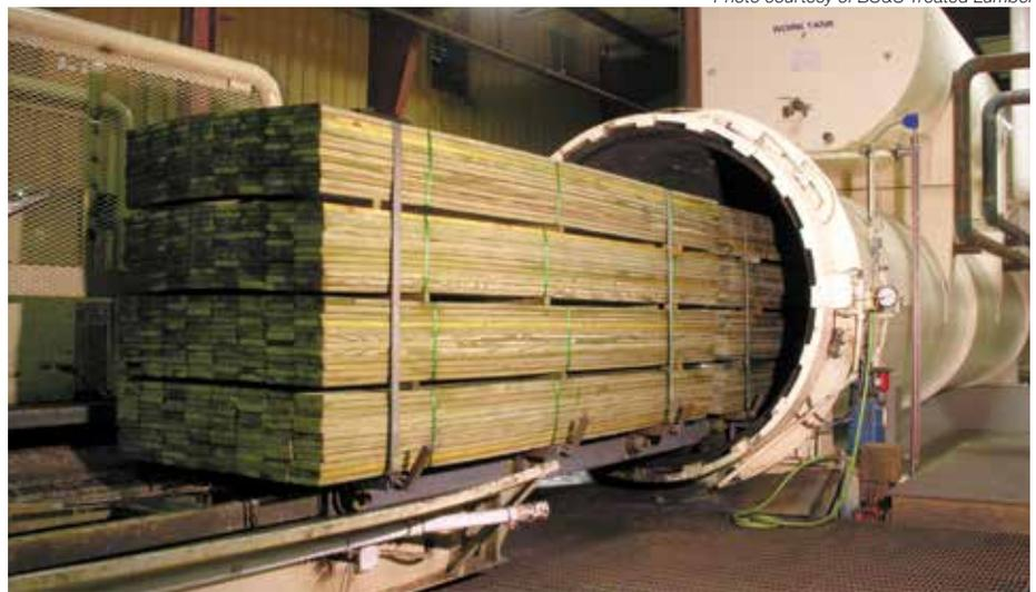
The IBC requires specific wood framing members of a building to be protected against decay and termites. Protection can be provided by using either naturally durable or preservative-treated wood.
