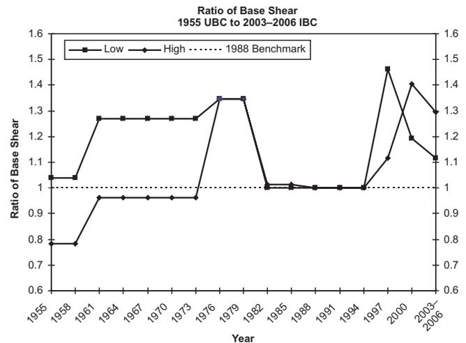
**Figure 2.**—Ratio of base shear to 1988 benchmark.
