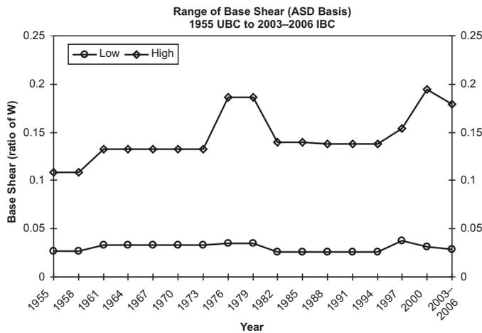
**Figure 1.**—Range of base shear, 1955 *UBC* to 2006 *IBC*.
