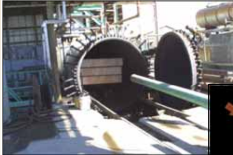
Untreated glulam in pressure cylinder ready for treatment
