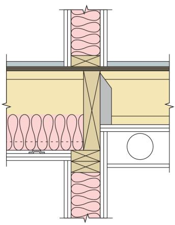
Other options for detailing this condition are given as exceptions to IBC 708.4. Exception 2 outlines a similar option but could also be seen to expand options for the ceiling including suspended ceilings, commonly used in corridors.
