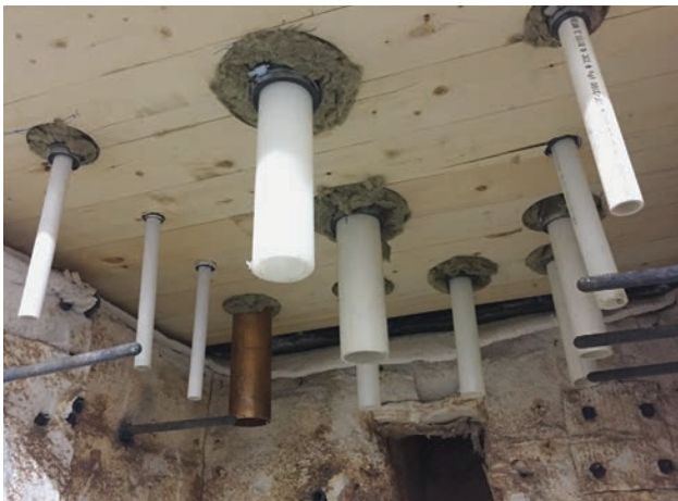
Exposed side of an assembly prior to a fire test
