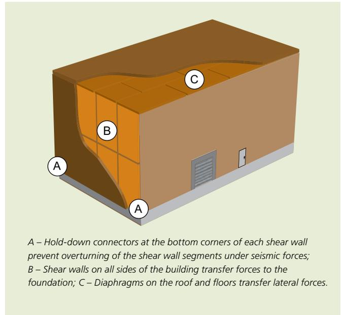
A – Hold-down connectors at the bottom corners of each shear wall prevent overturning of the shear wall segments under seismic forces; B – Shear walls on all sides of the building transfer forces to the foundation; C – Diaphragms on the roof and floors transfer lateral forces.
