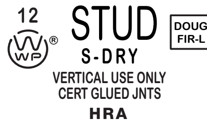
Fig. 1: Finger-jointed lumber joined with heat-resistant adhesives are marked with the designation HRA .
